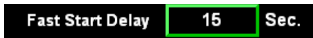
Figure 6 Setpoint Entry Box. The highlighted color reflects the user's security level. Green = access allowed, Orange = access denied.
