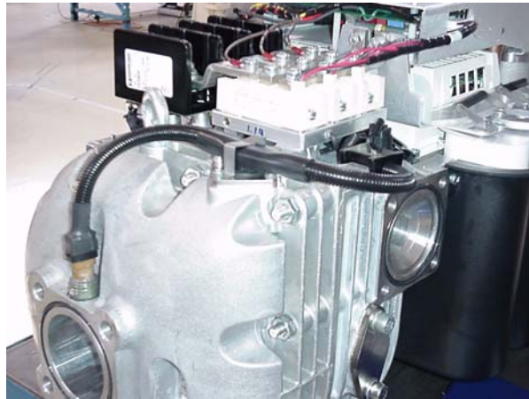
Figure 6-20 Cable Connection at the Suction Temperature/Pressure Sensor
