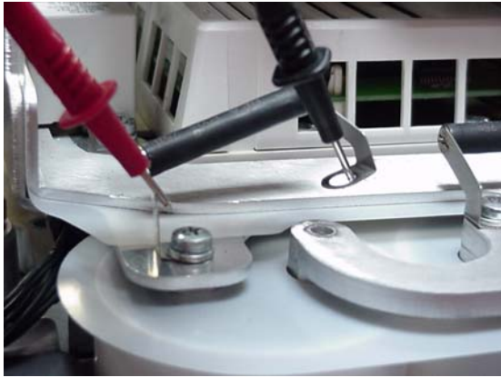
Figure 4-42 Resistor Resistance Measurement
