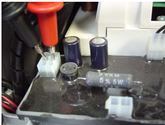
Figure 4-50 HV DC-DC Converter 24VDC Output Resistance Measurement
