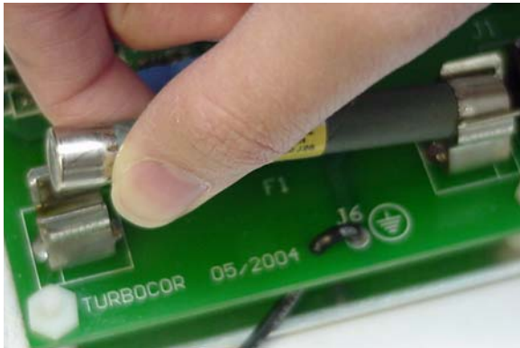
Figure 6-9 DC-DC Converter Fuse Removal
