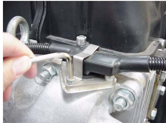
Figure 5-15 Disconnecting Power to the IGV Motor (1 of 2)
