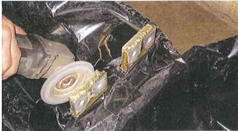
Plastic Bag and Tape keeps dirt out of Inductor
