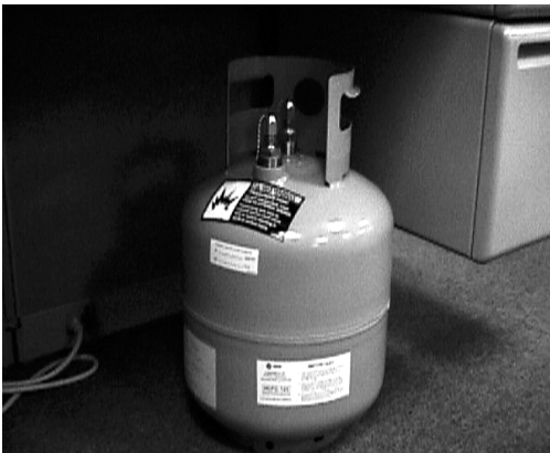
Figure 8 — Tank Label Location
