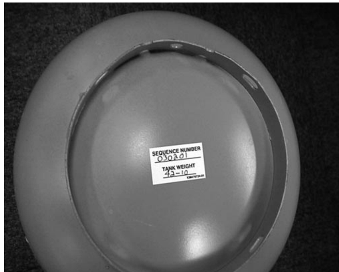
Figure 2 — Carbon Tank Tare Weight Sticker (Lbs.-Oz.)
