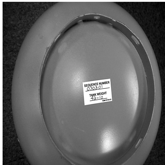
Figure 6 — Carbon Tank Tare Weight Sticker (Lbs.-Oz.)
