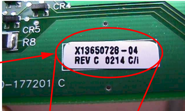
Figure 2 - Panel mounted LLID PCB date code example.
