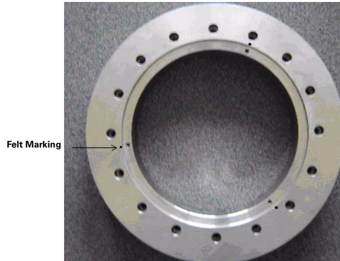
Figure 2. Orifice flange marking
