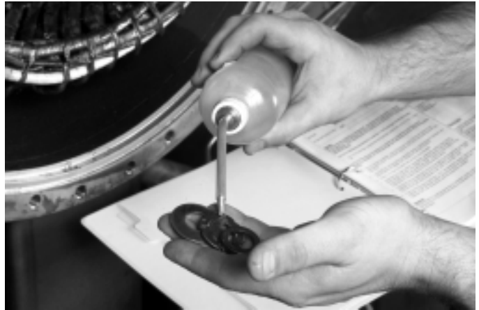
Figure 33. Lubricate the washer and direct tension indicator with OIL022 before installation on the cap screw.
