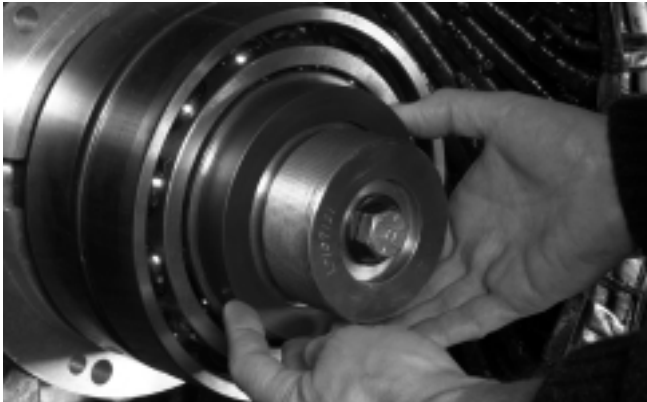
Figure 28. Install the hardened spacer ring as shown. The raised face of the ring goes against the bearing inner race.
