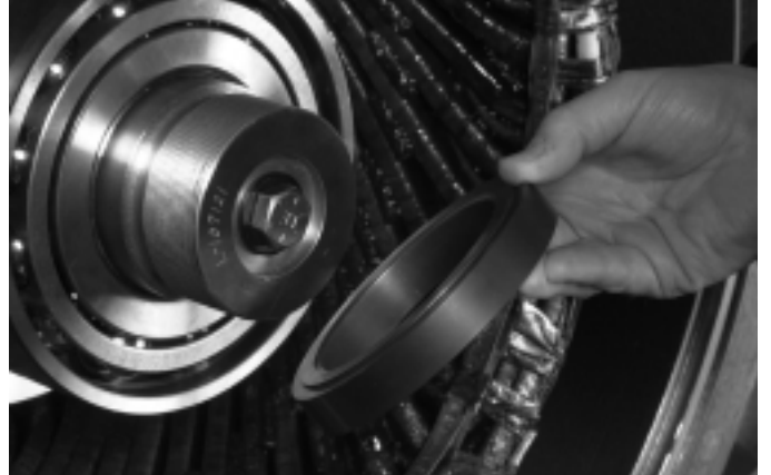
Figure 27. Install hardened spacer ring from TOL01550 with the raised face toward the bearings.
