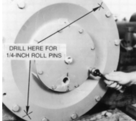
Figure 4. Removing bearing inspection plate
