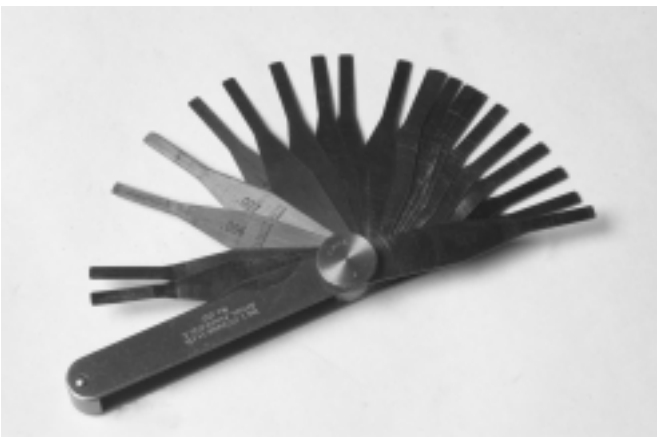
Figure 38. Narrow tipped feeler gauges. These are standard feeler gauges which were cut at the tips to allow measurement of the direct tension indicator clearance while torquing the cap screw. Note: KIT07314 provides similar gauges in .005, .010 and .015" - narrow tip.
