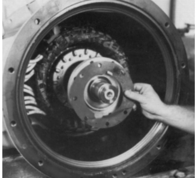
Figure 13. Inner bearing cap seal gasket - this gasket is not used on the center feed bearing design compressors.
