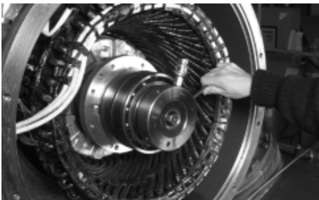
Figure 30. Hand tighten the hydraulic assembly nut using the rod provided with the nut.
