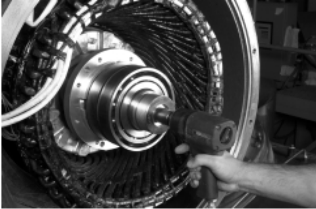
Figure 26. Use air impact wrench to tighten the cap screw on the shaft extension. Torque to 150 - 200 Ft. - Lbs.
