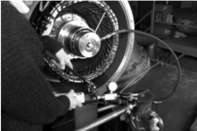
Figure 32. Pressurize the hydraulic assembly nut to 2700 to 2800 psi. Release the pressure at the pump and remove the hydraulic assembly from the shaft. Remove the hardened spacer and the shaft extension from the shaft.
