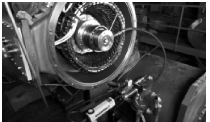
Figure 31. Bleed the hydraulic nut and hose assembly to remove all air from the system.
