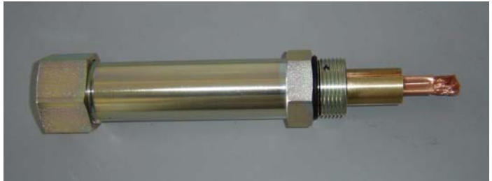
Figure 4. Original Bearing Inspection Cover without brush fitting or brush.
