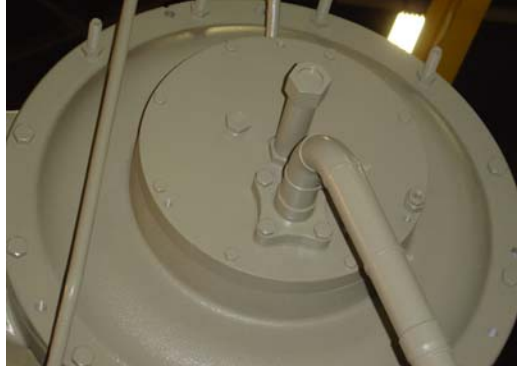
Figure 6. New design Bearing Inspection Cover with new design Grounding Brush installed.
