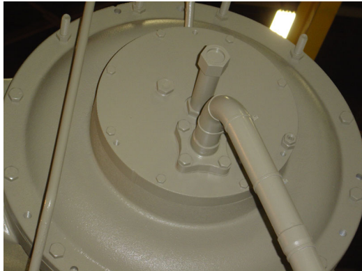
Figure 6. New design Bearing Inspection Cover with new design Grounding Brush installed.
