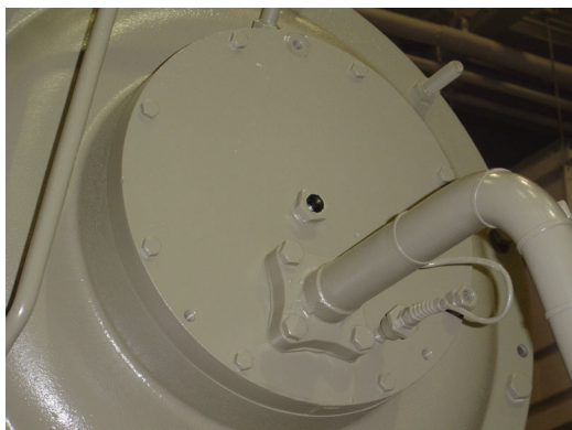
Figure 4. Original Bearing Inspection Cover without brush fitting or brush.
