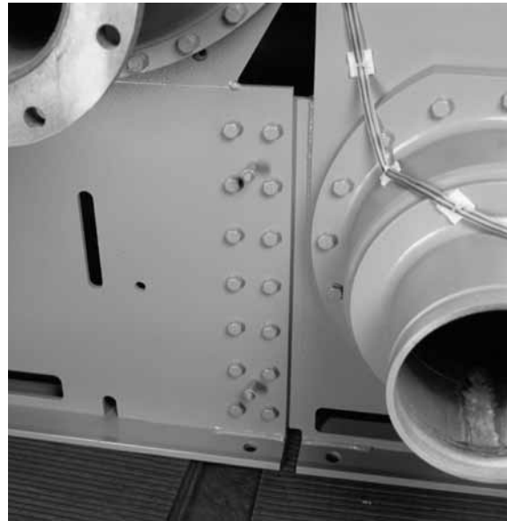
Figure 22. Separable shell unit (flange connection)
