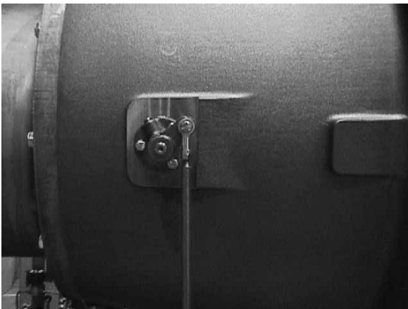
Figure 11. Vane actuator level on interstage
