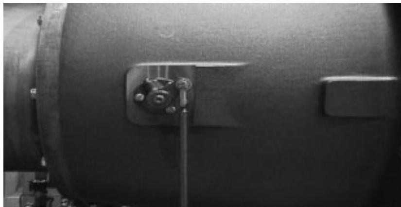
Figure 6. First stage vane operator lever on suction cover
