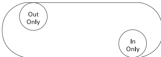
Large Two Pass Evaporator
