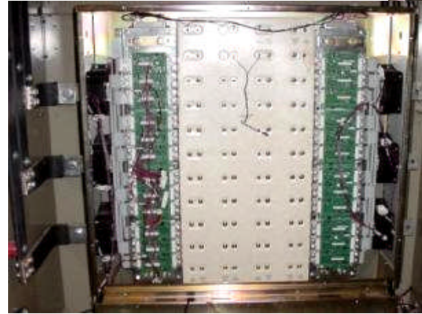
Second Layer View of Combined Power Board
