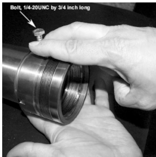
FIG. 3 – INSTALLING BOLT FOR SEAL REMOVAL
