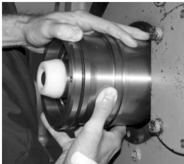
FIG. 14 – SEAL HOUSING SPACER INSTALLATION
