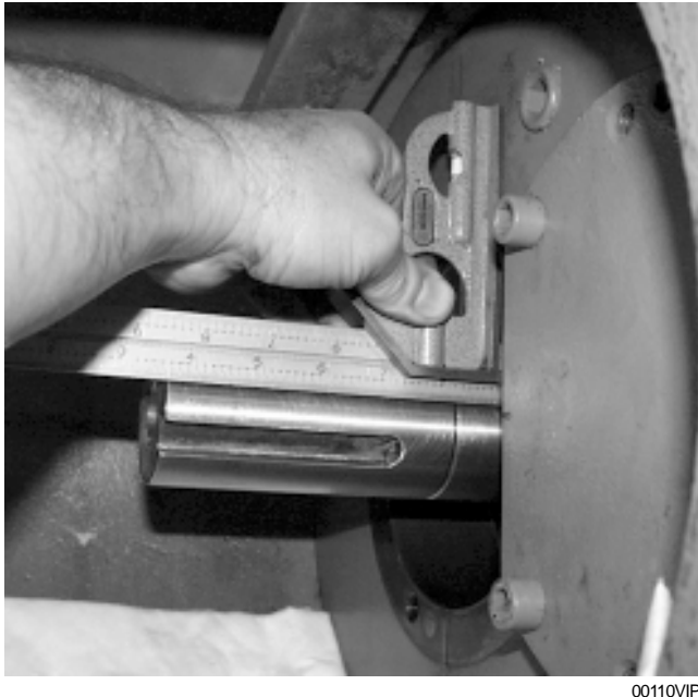
FIG. 8 – MEASURING SEAL OPERATING LENGTH
