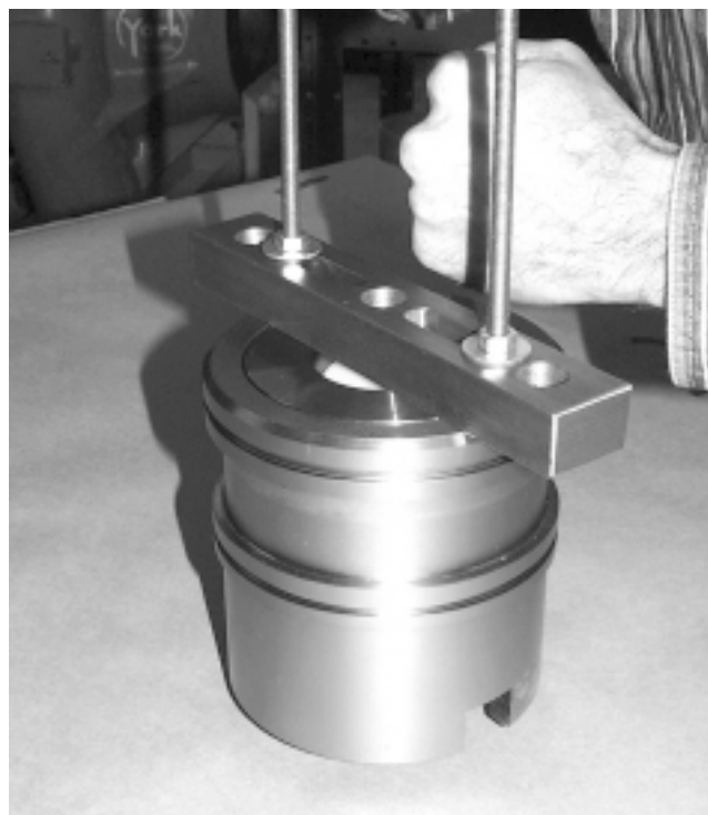
FIG. 13 – PUTTING SEAL HOUSING SPACER ONTO INSTALLATION TOOL
