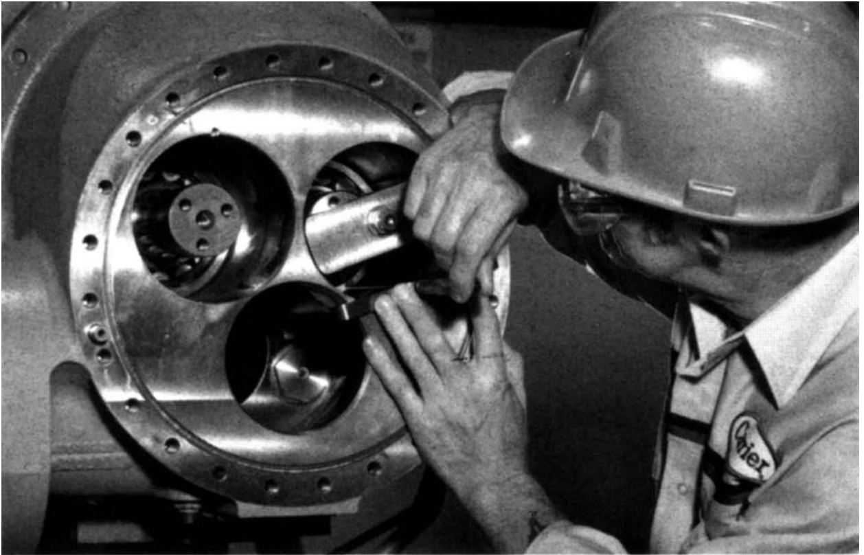
Figure 70 — End Clearance (Rotors)
