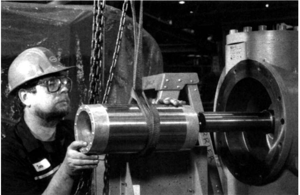
Figure 38 — Rigging the Rotor
