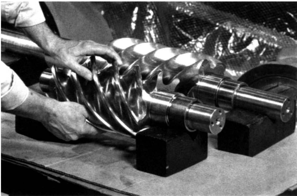
Figure 49 — Supporting Removed Rotors
