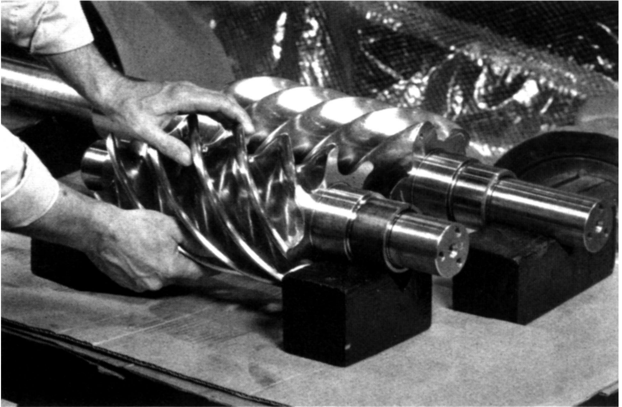
Figure 49 — Supporting Removed Rotors
