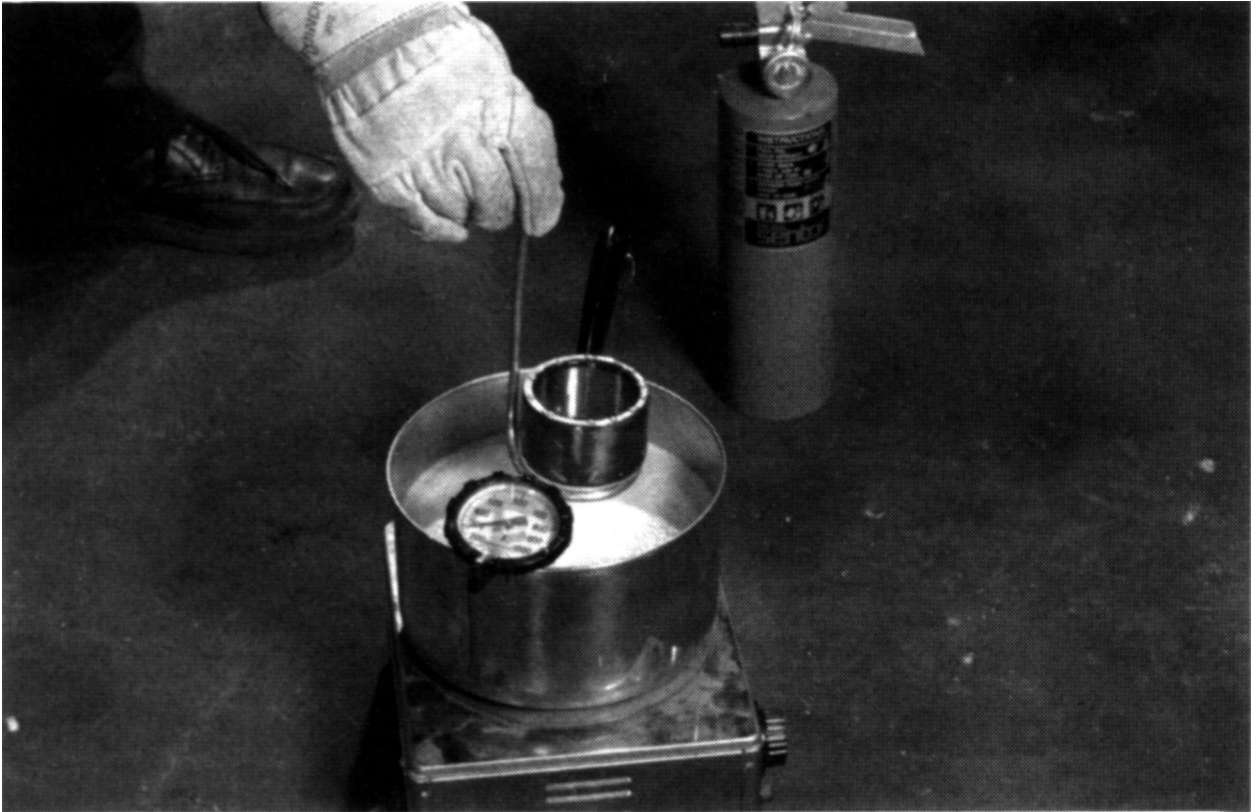
Figure 63 — Heating Roller Bearings
