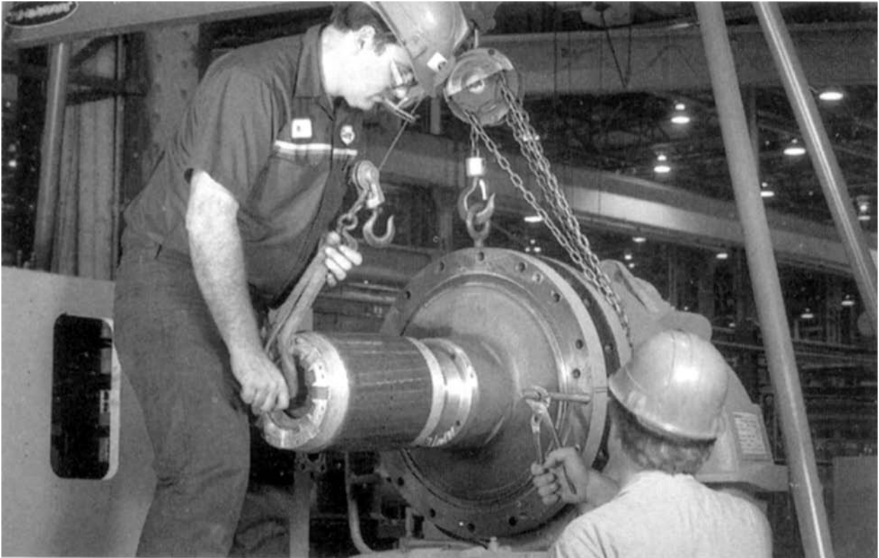
Figure 63 — Rigging the Transmission Case
