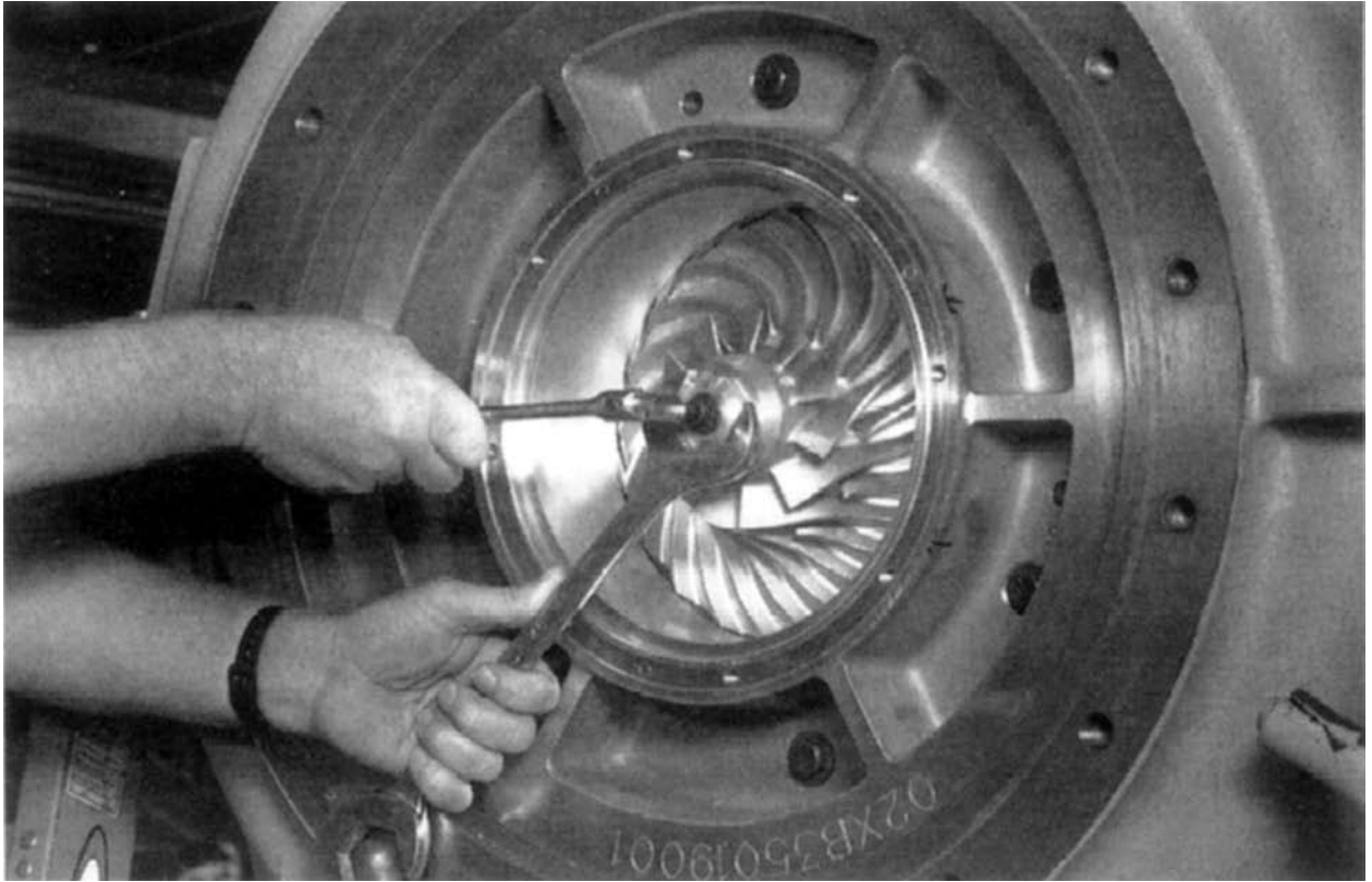
Figure 77 — Installing the Nose Piece
