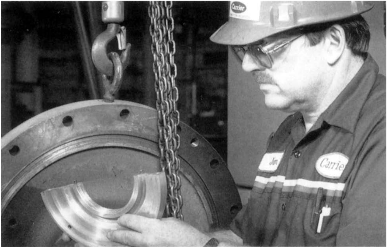
Figure 46 — Inspecting the Laby and Seal Ring
