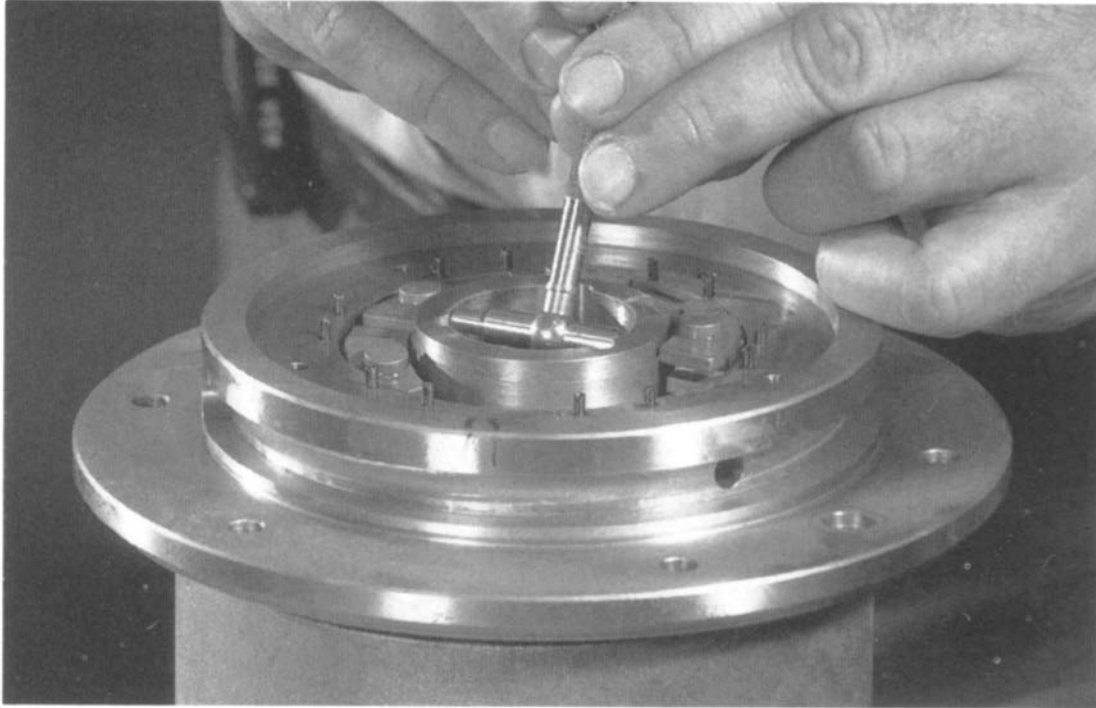
Figure 59 — Measuring the High Speed Main Journal Bearing Clearance
