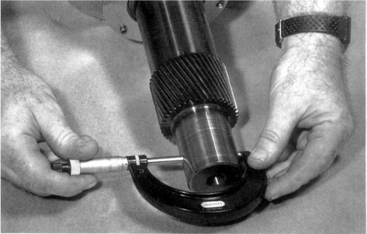
Figure 55 — Measuring the High-Speed Shaft Journal
