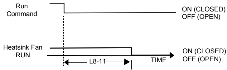
Fig. 84 Heatsink Cooling Fan Operation Timing Diagram
