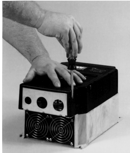
Figure 8: Removing Cover From 7.5 to 20 HP Inverters
