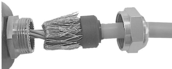
Fig. 132: Connect the shield in the cable screw fitting of the encoder
