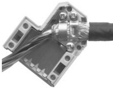
Fig. 131: Connect the shield in the sub D plug
