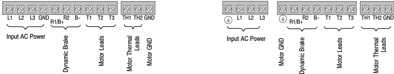
Figure 3-6 3 Phase Power Connections Size AA Enclosure Size B or C Enclosure
