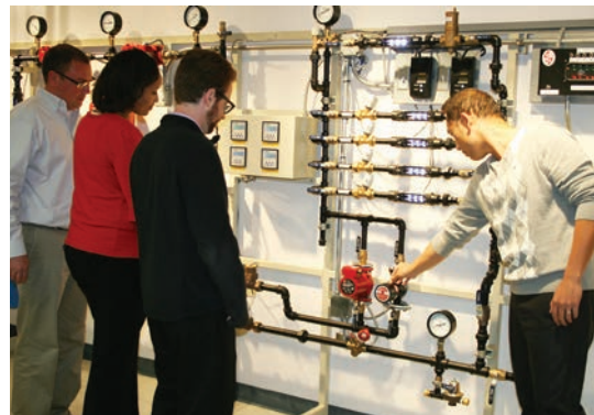
Primary-Secondary pumping demonstration.
