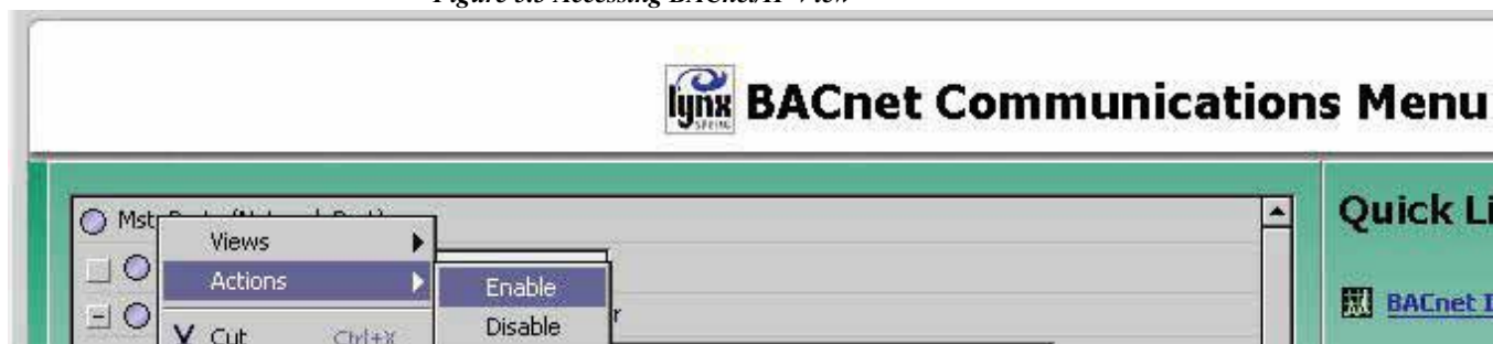
Figure 5.4 Enabling BACnet/IP Communications
