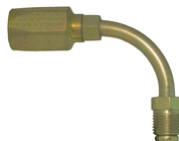
Inverted Male Swivel 90° Elbow Steel Reusable Fittings for SAE 100R5 Hose
