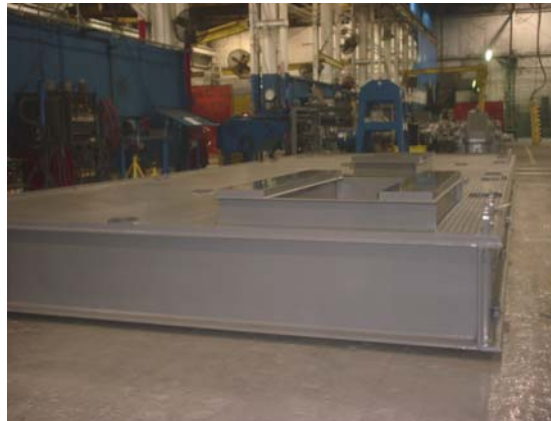
Leveled base at factory.
