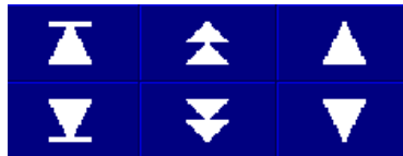
Figure 27 Alarm Navigation Box found on Alarm History and Active Alarms Screen
