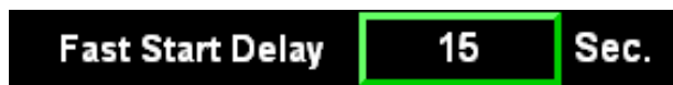
Figure 6 Setpoint Entry Box. The highlighted color reflects the user's security level. Green = access allowed, Orange = access denied.
