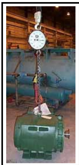
Figure 14. Weigh replacement motor
