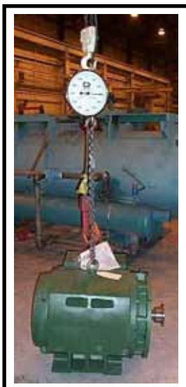
Figure 21. Weigh replacement motor
