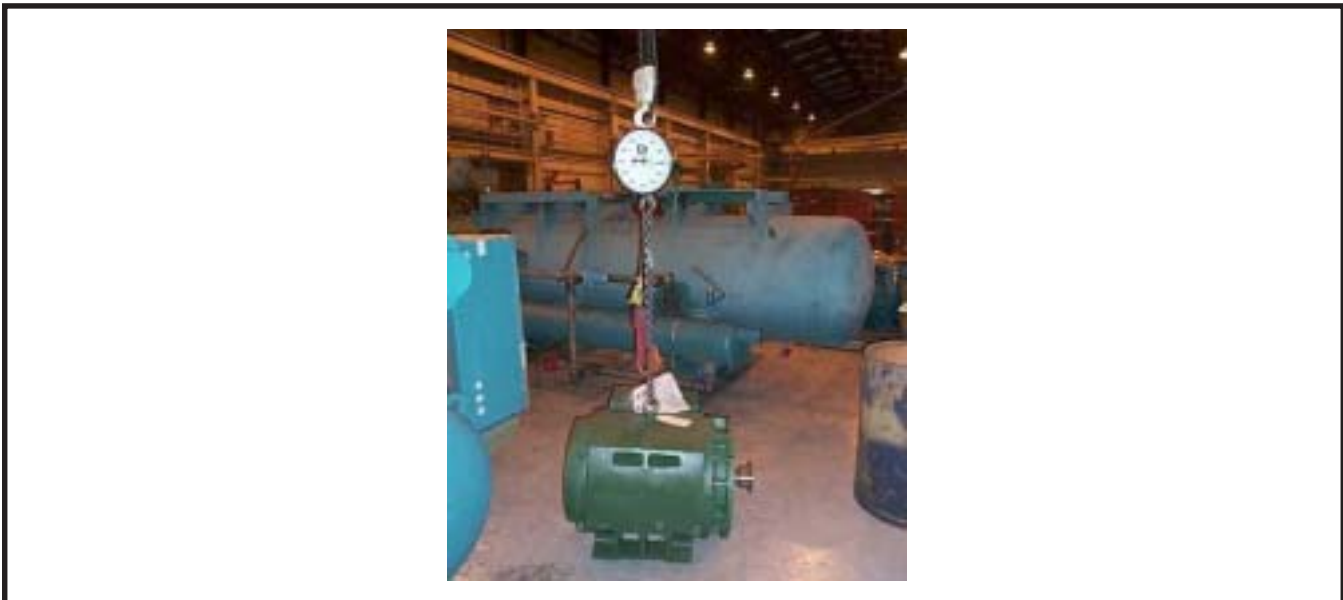
Figure 1. Weigh replacement motor.
