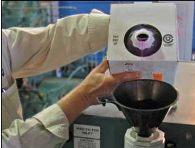
Figure 36 - Refilling the Cooling System
