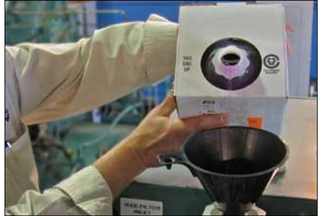
Figure 38 - Topping Off the Coolant Supply
