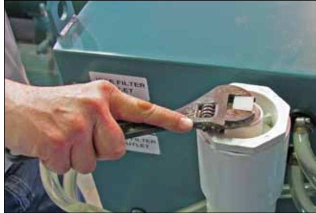
Figure 33 - Removing the Cooling System Pipe Plug
