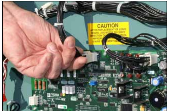
Figure 40 - VSD Logic Board Connection J2
