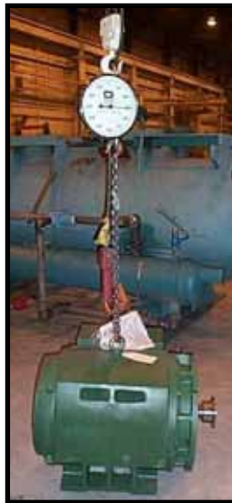
Figure 25. Weigh replacement motor (Contact the Baltimore Parts Center for a Hydraulic Pump Kit, p/n 720A0029G01 - Ph:800-336-7264)
