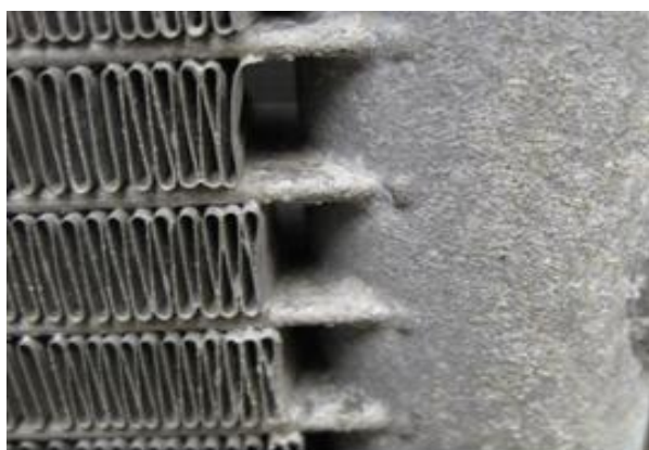
FIGURE 7 – Typical MCHX with Visible Flux Residue
