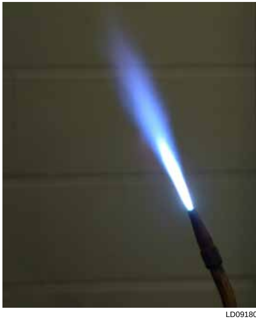
FIGURE 93 - PROPER TORCH FLAME FOR BRAZING
