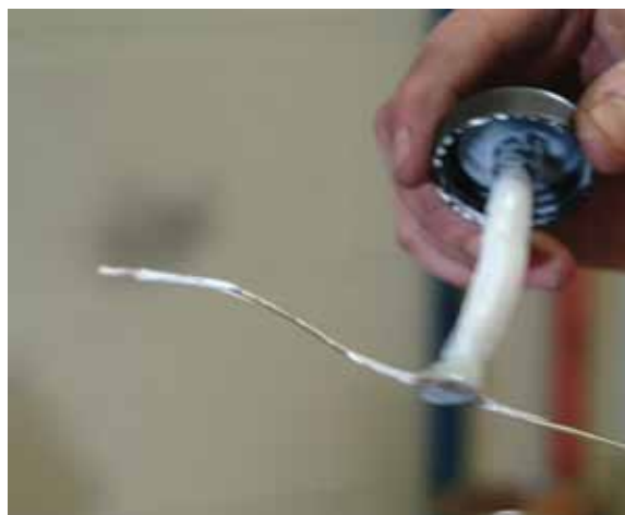
FIGURE 91 - APPLYING FLUX TO FILLER METAL
