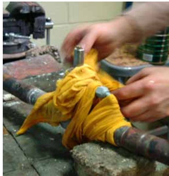
FIGURE 95 - USING WET CLOTH TO PROTECT COMPONENTS WHILE BRAZING
