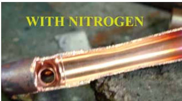
FIGURE 84 - PIPE BRAZING WITH NITROGEN
