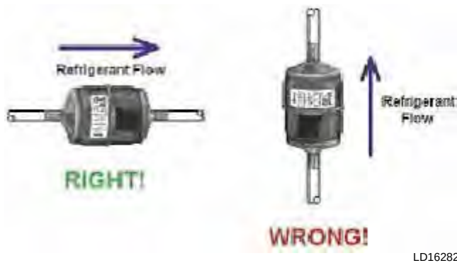
FIGURE 74 - FILTER DRIER INSTALLATION
