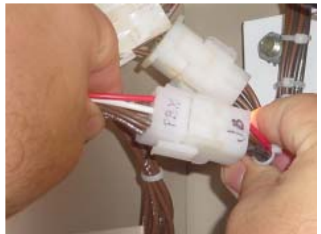
FIG. 12 - CONNECTING SMART RELAY HARNESS
