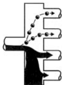
FIG. 22 – POOR REFRIGERANT/VAPOR DISTRIBUTION
