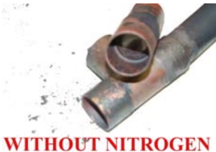
FIG. 8 - PIPE BRAZING WITHOUT NITROGEN
