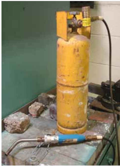
FIGURE 79 - HAND HELD TORCH AND TANKS
