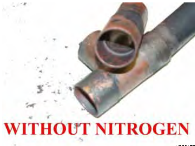
FIGURE 85 - PIPE BRAZING WITHOUT NITROGEN
