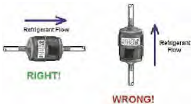
FIGURE 74 - FILTER DRIER INSTALLATION
