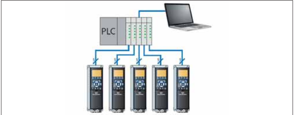
Fig. 8.7 Traditional wiring. No fieldbus
