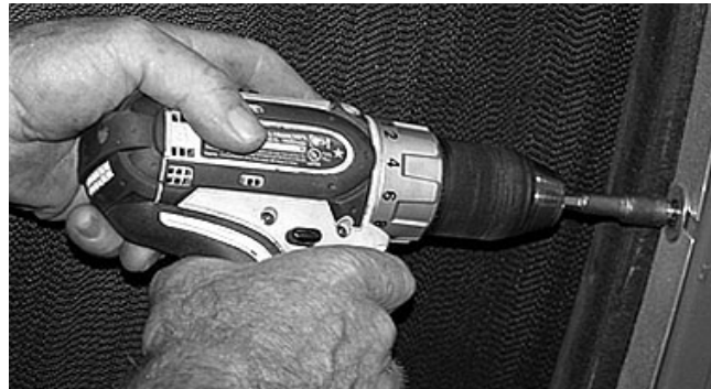
FIGURE 75 - LOOSEN SCREWS BEFORE ADJUSTING SEALS
