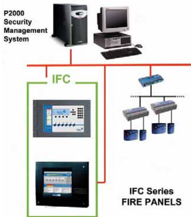
Access Control to Fire Detection Systems Integration
