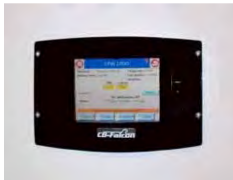
Figure B9-6. CB Falcon Display/Operator Interface
