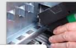
Insert the 1771 swing-arm with attached field wires to the conversion module.
