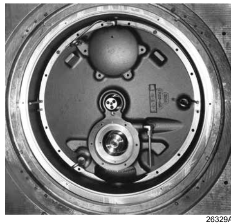
FIGURE 36 - ALL FRONT END BEARING REMOVED
