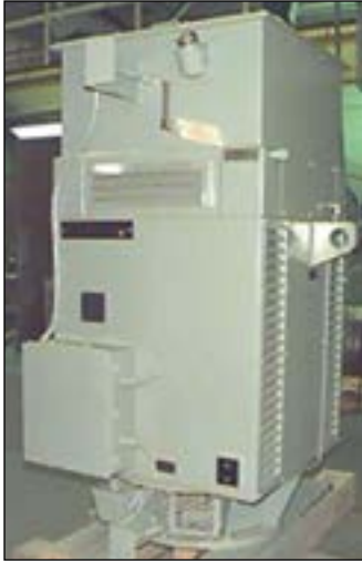
HP: 350 RPM: 1800 Frame: V5830 Enclosure: DPG Application: Moderator Pump Industry: Nuclear Generating Station
