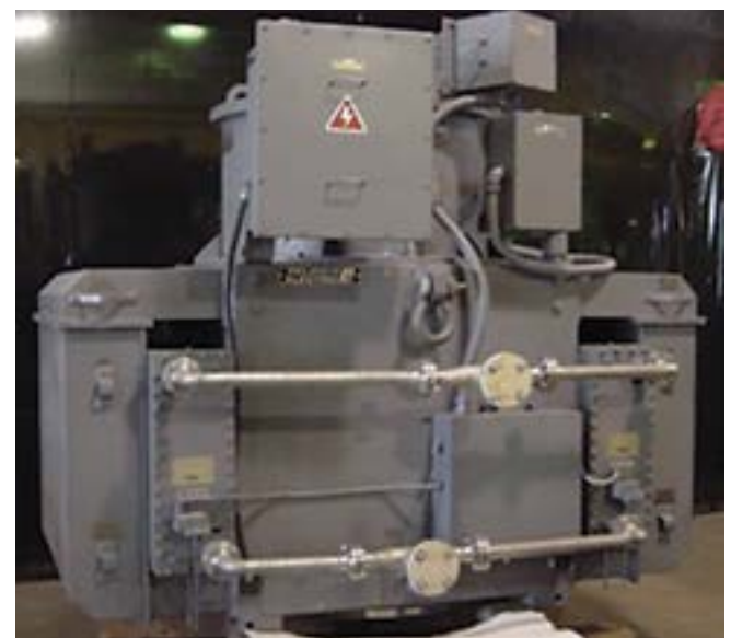
Dual TEWAC exchanger hoods
