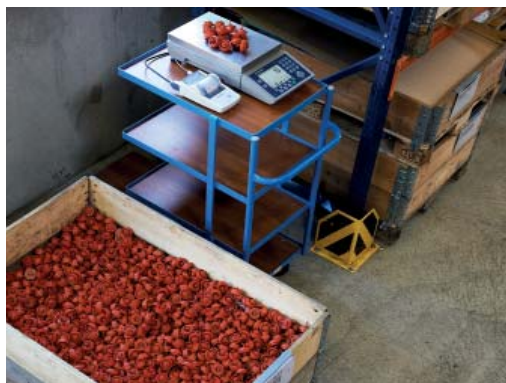
Up to four scales can be connected to a versatile counting terminal with large display and keyboard for error-free operation and barcode scanner/printer to properly identify/mark all components.
