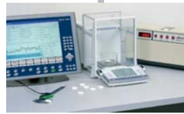
Testplace module with weighing station, tablet tester and dimension measurement
