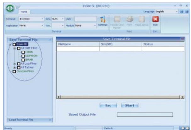
As this IND780 example shows, InSite® SL supports the selection of specific configuration and data files when saving
