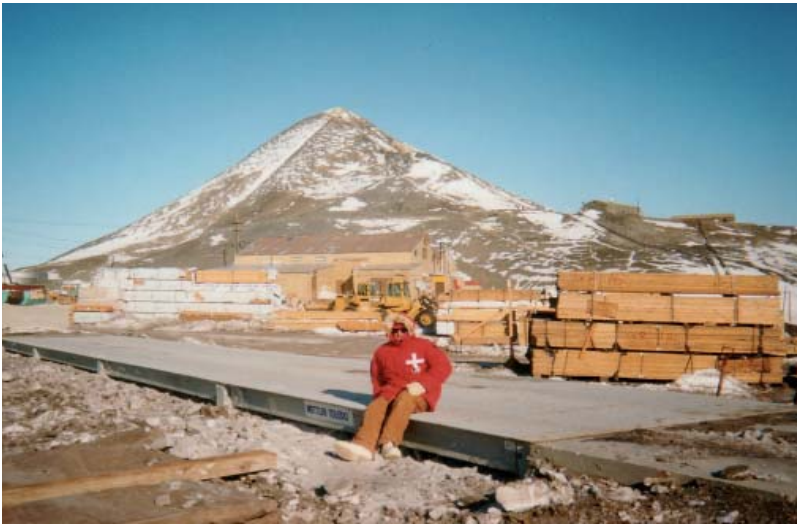
METTLER TOLEDO scale installed at McMurdo Station, the only truck scale in Antarctica (Average temperature -17°C)
