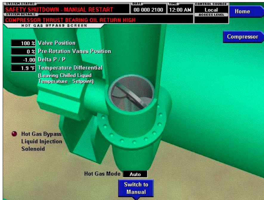
FIGURE 9 - HOT GAS BYPASS SCREEN
