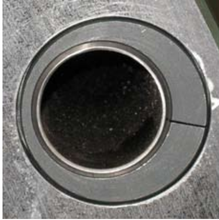
FIG. 4 – INSTALLED TUBING CLAMP
