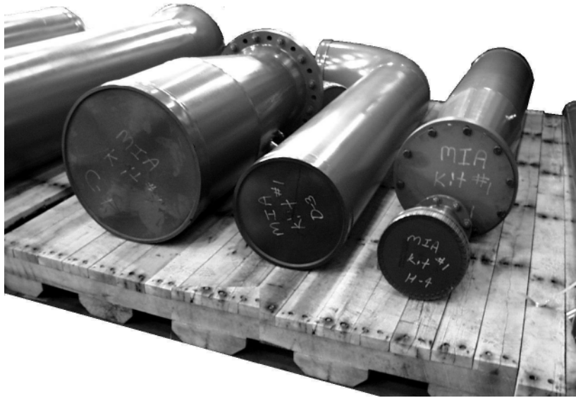
FIG. 13 – PARTIAL PREFABRICATING PIPING
