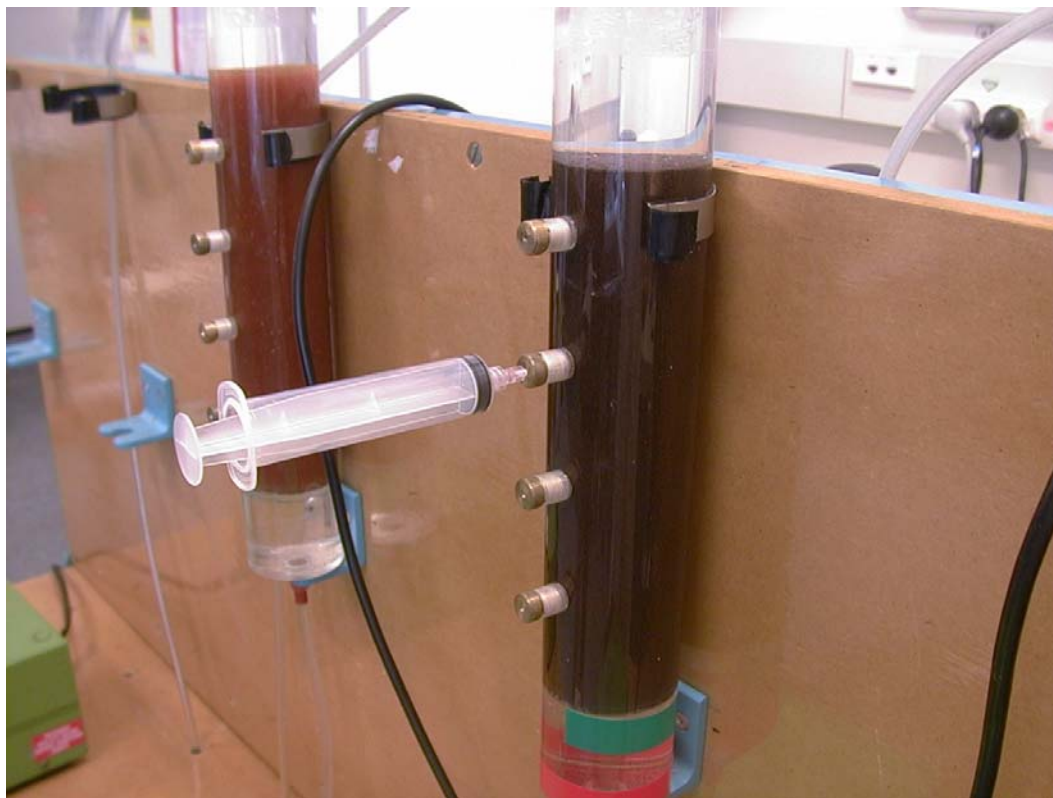
Figure 3.4: Column sample point.
